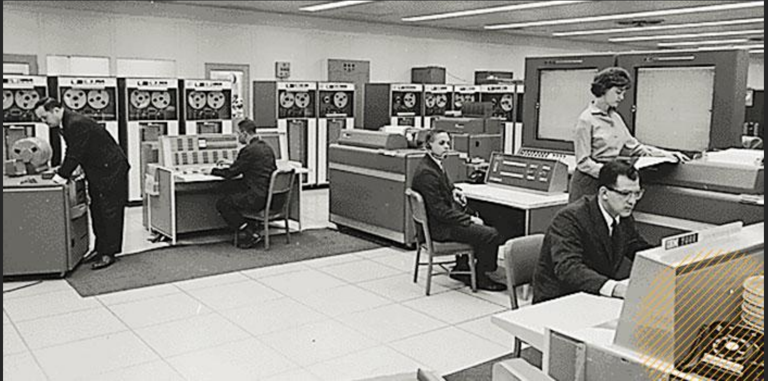
Above: Workers and the IBM 7094, early 1960s. It helped NASA in the Apollo and Gemini programs, as well as being used by the Air Force in an early missile defense system.
